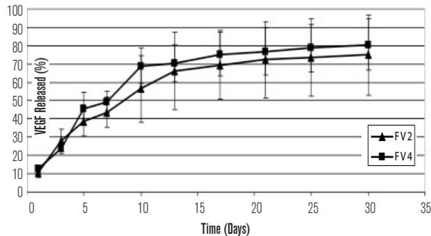
**Figure 3.** In vitro release profiles of VEGF from VEGF loaded PLGA microspheres prepared with 10 µg VEGF and 2% (w/v) concentration of PVA as an aqueous inner phase (FV2) and VEGF loaded PLGA microspheres prepared with 10 µg VEGF and 1% (w/v) concentration of PVA as an aqueous inner phase (FV4) in pH 7.4 phosphate buffer solution for 1 month at 37°C. Data represents the mean±S.D. (n=3).
